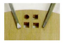
FOUR-SQUARE • After drilling the holes, use a 1/8" chisel and a triangular file to clean up the hole. The top left hole is shown after drilling, while the two lower holes have been completed.
